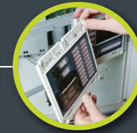
Fully interchangeable indicator modules
